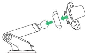
Connect the Mount Cradle with the Ball Joint.
