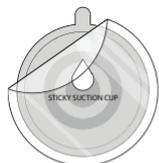
Peel off the protective film on the Suction Cup and press mount firmly onto the dashboard pad.
