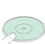
Peel off the film on the dashboard pad & stick on the desired installation location.
