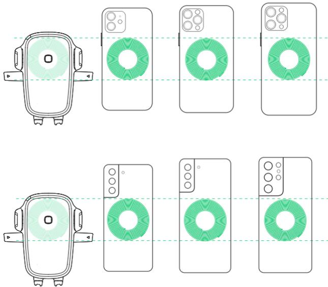
! For optimal wireless charging, please make sure your smartphone and mount's Qi coils are aligned.
