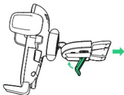
2. Put the mount into the CD slot and pull the lever to lock it into place.
