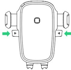
2. Press your device against the Easy One Touch trigger button. The mount's arms will automatically close on contact for a secure hold.
