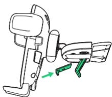
3. Test to make sure the mount is secure. Insert bracket only if needed.
