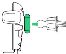
1. Attach the air vent mount to the cradle. Tighten using the adjustment knob.
