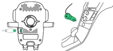
! The Easy One Touch Wireless 2 is powered by a micro USB cable. There is no on/off switch on the mount. Once it is plugged in, the mount will remain on until the vehicle is turned off.
