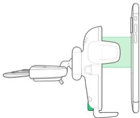
4. Align your smartphone in the center of the Easy One Touch trigger button. The indicator light will turn on when the phone is successfully charging.
