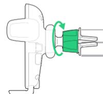
2. Loosen the twist lock and push the mount completely onto the air vent blade.
