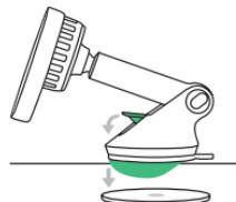
3. Push down the locking lever to engage suction.
